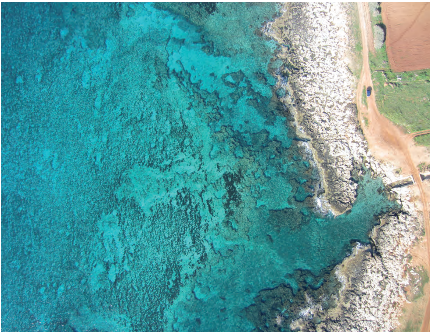
▲ UAV images are used to derive the bathymetry in shallow clear, calm waters and seabeds with texture.
